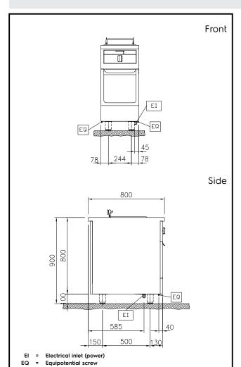
Electric Supply voltage: 400 V/3N ph/50/60 Hz Total Watts: 10 kW **Key Information:** Number of wells: Usable well dimensions (width): 240 mm Usable well dimensions (height): 225 mm Usable well dimensions 380 mm (depth): Thermostat Range: 100 °C MIN; 180 °C MAX External dimensions, Width: 400 mm External dimensions, Depth: 800 mm External dimensions, Height: 800 mm Net weight: 65 kg On Base;One-Side Configuration: Operated Sustainability
